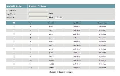
The switches provide Port Control Rate Limit, including Ingress and Egress Rate Limit.
