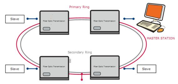
If primary fiber is lost, data is passed onto the Secondary ring to maintain the ring integrity  $% \left( 1\right) =\left( 1\right) \left( 1\right)$
