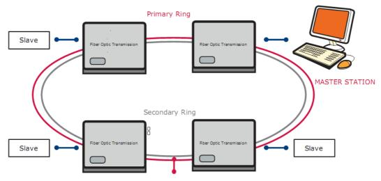
If primary fiber is lost, data is passed onto the Secondary ring to maintain the ring integrity
